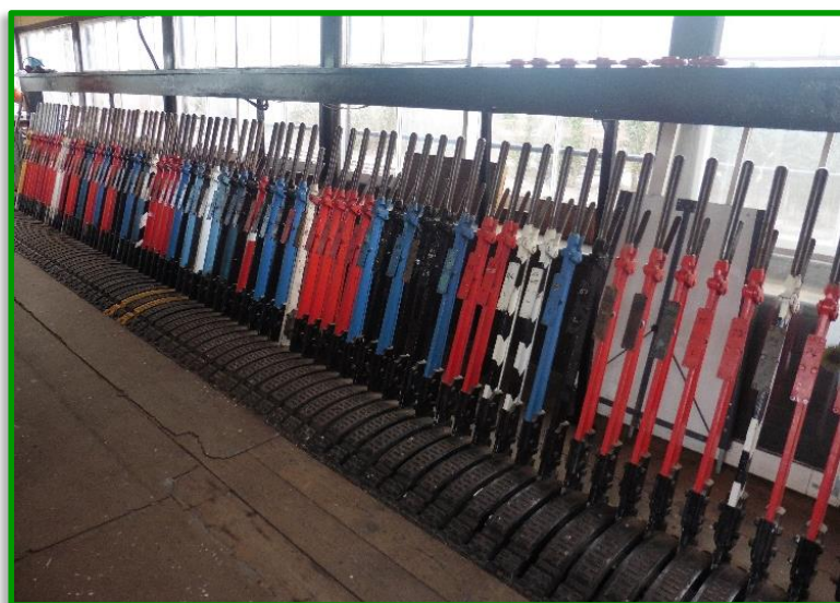
Photo above – Part of the 1964 illuminated diagram which will be used by the simulator. Photo left – The 81 levers to form the simulator.
